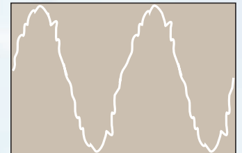
12-pulse input with phase-shift transformer.
